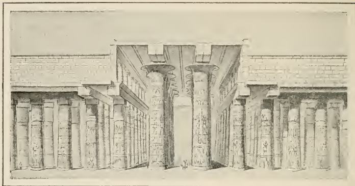
FIG. 238.—TRANSVERSE SECTION OF THE HYPOSTYLE HALL AT KARNAK (After Chipiez) ( Hist. de l'Art. vol. I, pl. V).
